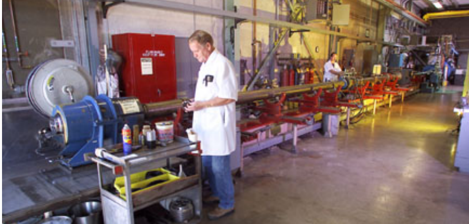
1) Two-stage gas gun (Livermore) 20 GPa in deuterium
